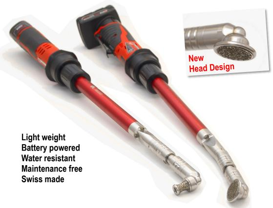
T-0100: Motor: The Terafloat uses a 12V Milwaukee motor with a variable speed trigger. The motor features an electronic shut-off protection when the grinding disk is blocked. The motor is fitted with powerful M12 Li-ion batteries, (standard 2.0Ah or optional 4.0Ah), and it has a LED light indicator for the remaining charge of the batteries. The basic sets use a single battery charger and the standard set a four-bay charger. A dual wall/car charger is available.
